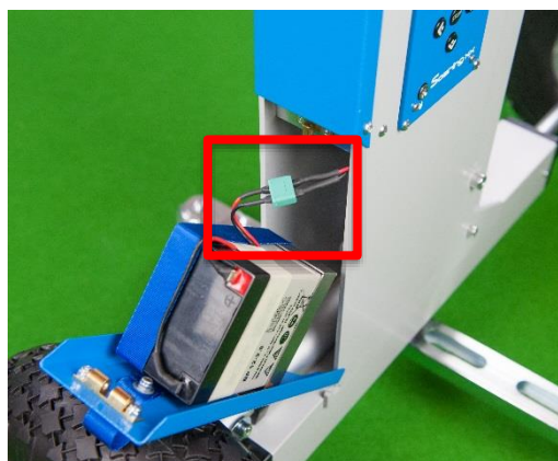
Figure 15: Showing the way of connecting the battery to the control unit.
