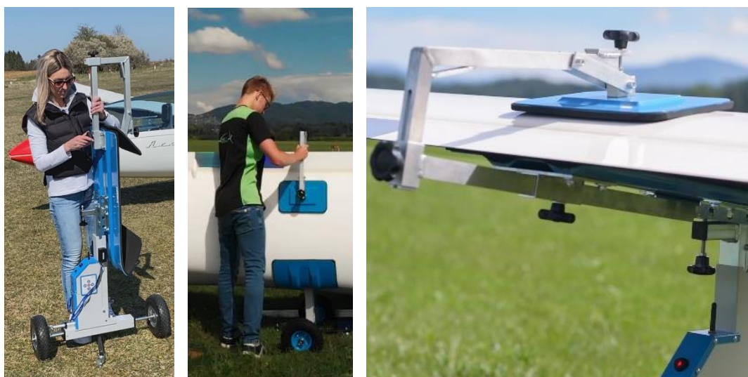
Figures 23 - 25: Showing a secured wing with a locking arm.
