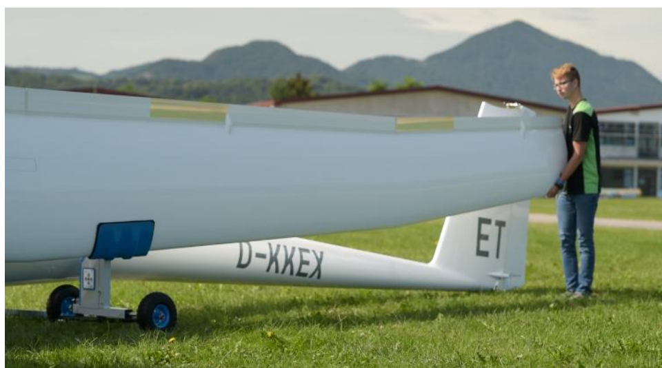
Figure 22: Showing a properly balanced wing in a wing-holder.
