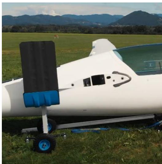
Figure 21: Rigging system positioned next to the fuselage.
