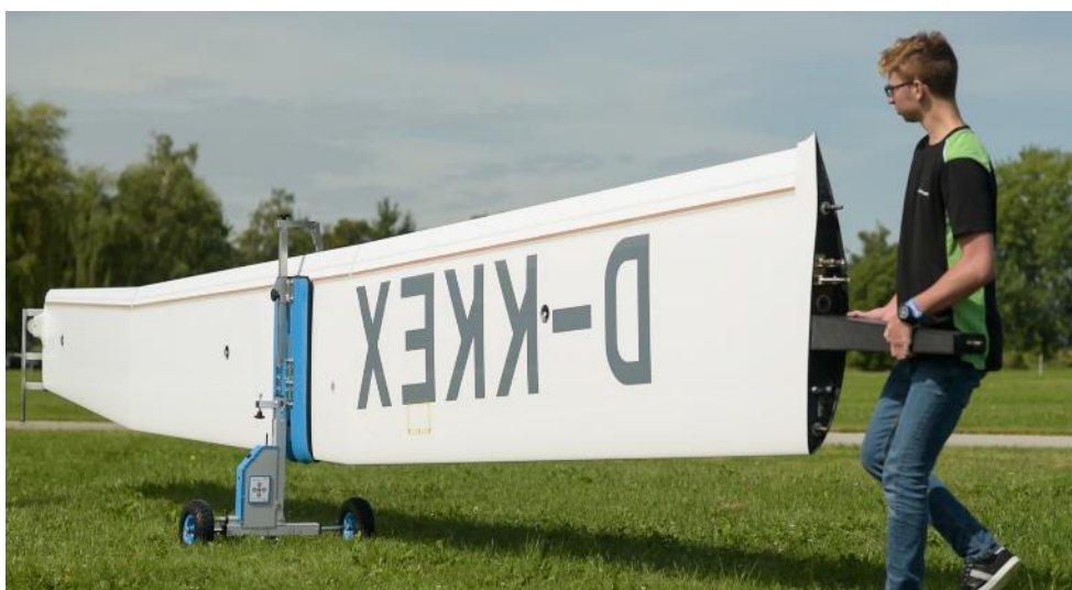
Figure 26: Moving of the wing for inserting it into the fuselage.
