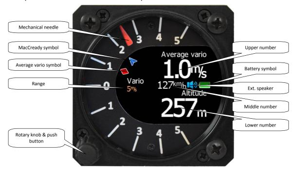
**Mechanical needle** displays vario. Printed scale can be chosen (when ordered) in the range of -5 to 5 or from -10 to 10. Within the software the range can be set to 2.5, 5, 10m/s or 5, 10, 20kts or 500, 1000, 2000fpm.
