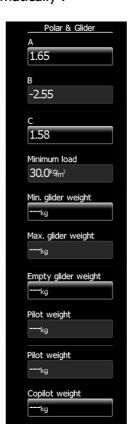
Polars for most modern gliders are already prepared. Use Glider type control, to list between preloaded glider polars.
