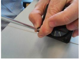
Remove rotary knob cap with a knife or flat screw driver, then hold knob and unscrew it. Remove remaining three screws. Install V3 into the panel, screw back all screws and knob. Make sure that between knob and panel is some space, to push button.
