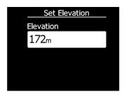
The instrument will offer elevation over standard pressure level QNE. Use the knob to finetune the elevation.
