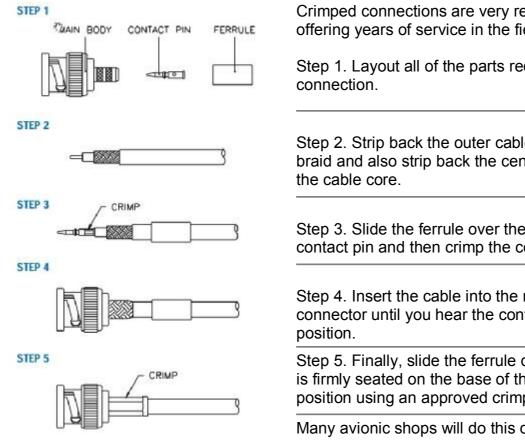
Crimped connections are very reliable and strong offering years of service in the field.
