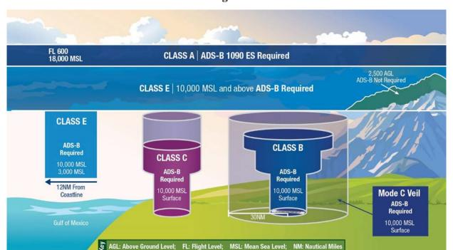
Figure 3-1. Automatic Dependent Surveillance-Broadcast Airspace Rule (§ 91.225)
