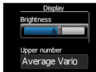
With push button you can activate slider control, then with rotation of the knob you can select the preferred value and confirm it with the push button.
