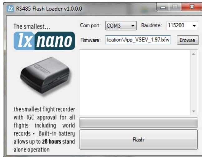
4. Choose correct **serial port** and baud rate (**115200bps**)
