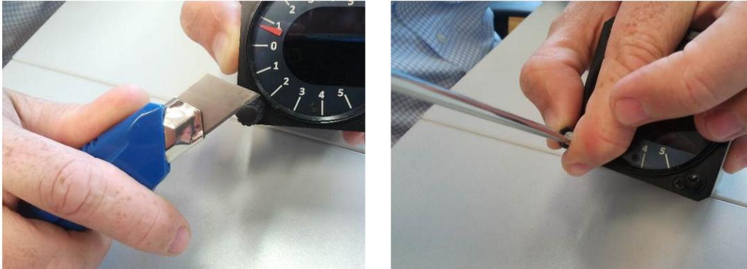
Remove rotary knob cap with a knife or flat screw driver, then hold knob and unscrew it. Remove remaining three screws. Install V3 into the panel, screw back all screws and knob. Make sure that between knob and panel is some space, to push button.
