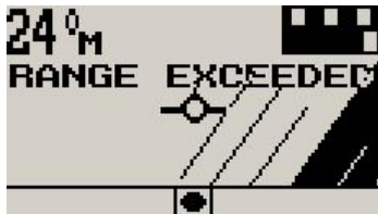
Message displayed when the maximum bank, pitch or yaw rates have been exceeded
